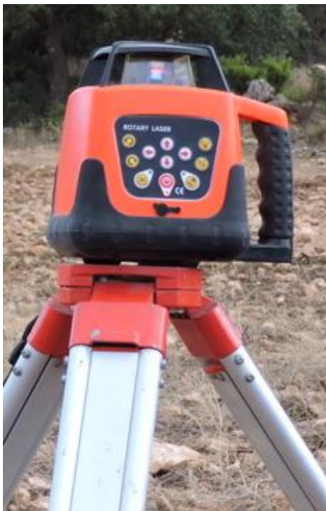
A swale laser is used to place poles to indicate where the swale will be made
